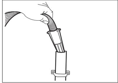
4. **To a stand pipe with vent-hole** - Insert the drain hose directly into a drain pipe. Refer to the illustration.
