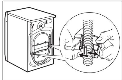
7. Remove the three transit bolts and pull out the plastic spacers.
