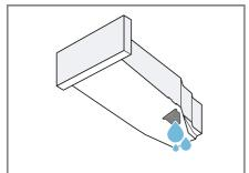
Check the condensation container filter → Page 44 regularly and clean the filter if it is dirty. Make sure that you insert the condensation container before operating the appliance.
