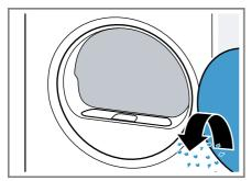
3. Remove the two-part fluff filter.
