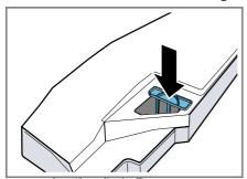
5. Insert the condensation container. → "Inserting the condensation container", Page 33
