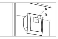
Before switching off the appliance, remember to turn off the fan by pressing the button (A). The green light (B) disappears.
