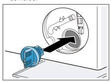
5. Screw on the pump cap.
