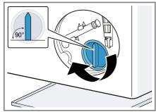
The handle on the pump cap must be in a vertical position.
