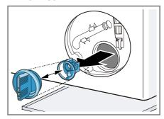
**2.** Clean the interior, the thread on the pump cap and the pump housing.
