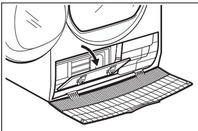
5. Catch the handle and pull the condenser out from the bottom compartment. Move condenser horizontally to avoid spilling any remaining water.
