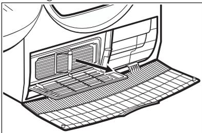
6. Clean the condenser in vertical position over a basin. Rinse through with a hand shower.
