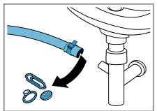
Reattach the water outlet hose and secure the connection point using the hose clamp.
