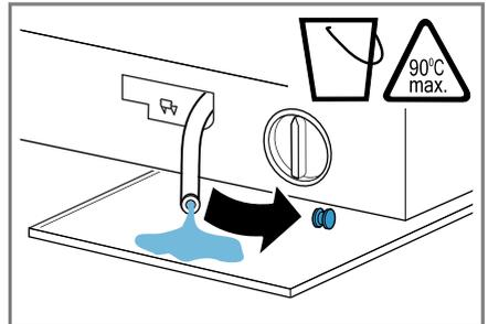
8. Firmly press on the sealing cap.
