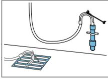
Fix and secure the water outlet using an elbow.
