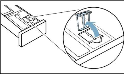
2. Remove the stopper inserted in the recess on the condensation container.
