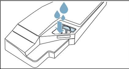
**Note:** Hold the full condensation container horizontally at all times so that no liquid spills out.
