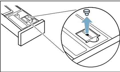
3. Turn the condensation container 180° onto its underside and insert the stopper.
