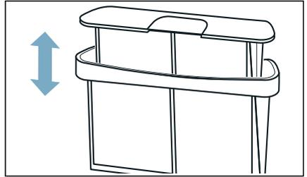
5. Open the two parts of the filter.
