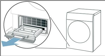
7. Rinse the insert under running water and dry it off.
