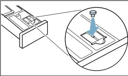
10. Pull the filter out of its snap-in lock.
