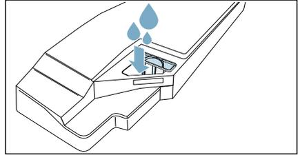
**Note:** Hold the full condensation container horizontally at all times so that no liquid spills out.
