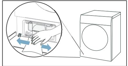
3. Unlock the levers on the heat exchanger cover.
