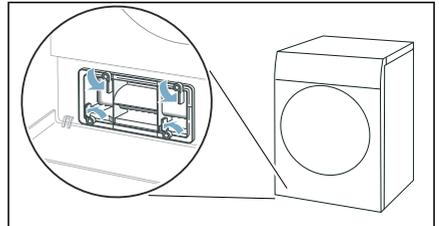
4. Pull the heat exchanger cover out by its grip.
