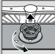
Rotate filter cylinder, remove filter system ...
