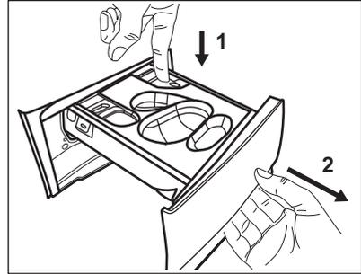
2. Remove the container for liquid detergent, if inserted.
