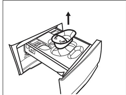
3. Lift up the top cover of the compartments to remove it.
