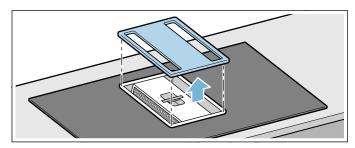
2. Remove the metal grease filter and container.
