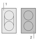
**Note:** In the combi zone, the PowerBoost function can only be activated if the two hotplates are used independently of each other.
