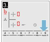
**Note:** After eight minutes, the appliance automatically switches back to fan setting  $\mathfrak{F}$ .
