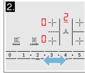
3. To set a different setting, touch the ♣ symbol and select the required setting from the setting area. The setting that is selected will be displayed.
