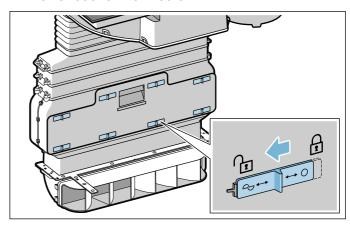
Open the drawer in the flat duct and remove the activated charcoal filter.
