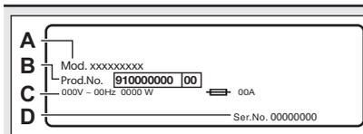
The rating plate **6** reports the model name (**A**), product number (**B**), electrical ratings (**C**) and serial number (**D**).
