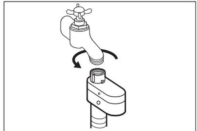
**!** **WARNING!** The inlet water shall not exceed 25 °C.
