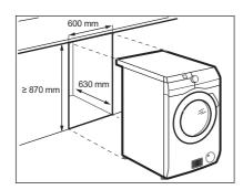
The appliance can be installed as freestanding or below the kitchen counter with correct space (see picture).
