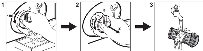
Clean the filter regularly and, especially, if the alarm code **E2** appears on the display.
