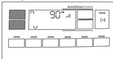
6. After about 10 seconds the display returns to the programme information screen or hold pressed the Temp. and the Spin buttons again to exit immediately.
