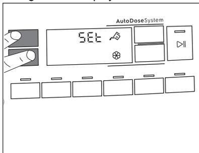
4. Touch related tank buttons to toggle function off and on. The display shows OFF when a tank is disabled or shows tank indicator when it is enabled.
