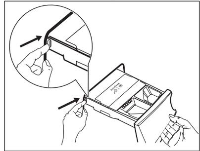
2. Remove the insert for the softener and, if inserted, the container for liquid detergent.
