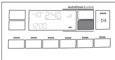
5. To set basic dosage touch related tank buttons until default dosage laundry product and two arrows on bottom of display appear. Touch the Temp. button repeatedly to adjust the dosage upwards and the Spin button
