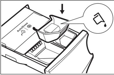
**i** When using liquid detergent, make sure that the **special container for liquid detergent** is inserted. Refer to the "Manual filling the detergent and additives" paragraph in this chapter. The liquid detergent container is supplied inside the drum.
