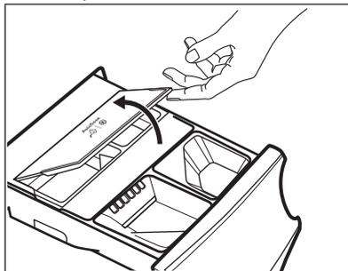
3. Gently pour only liquid detergent in the AutoDose detergent tank
