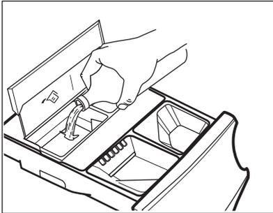
4. Gently pour only liquid softener in the AutoDose fabric softener tank
