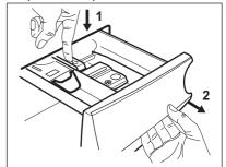
Remove the top part of the additive compartment to aid cleaning and flush it out under running warm water, to remove any traces of accumulated detergent. After cleaning, put the top part back into position.
