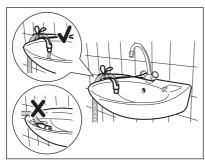
Make sure that the plastic guide cannot move when the appliance drains and the drain hose end is not immersed in the water.
