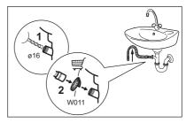
Connect the drain hose to the spigot and tighten it with a clamp. Make sure that the drain hose makes a loop to prevent particles going into the appliance from the sink.
