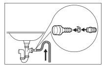
Make sure that the drain hose makes a loop to prevent particles going into the appliance from the sink.
