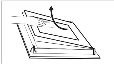
4. Clean the door glass panels. To install panels, do the same steps in reverse.
