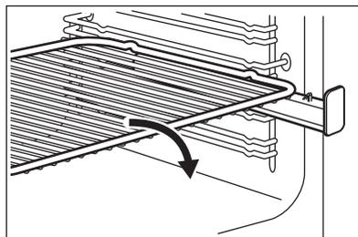
Put the wire shelf on the telescopic runners so that the feet point downwards.
