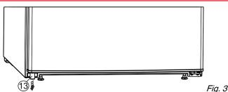
Remove the spacer Fig. 3 (13) from under the left-hand side of the door.
