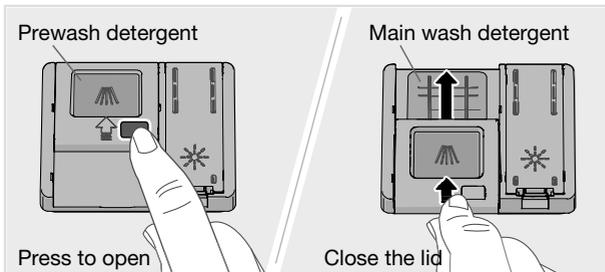
The detergent compartment must be dry when adding detergent. There is one compartment for the prewash and one for the main wash. If dishwasher detergent powder or dishwasher detergent gel is used, you can add a small amount of the detergent to the prewash compartment. Contact the detergent manufacturer if you have questions about the detergent.
