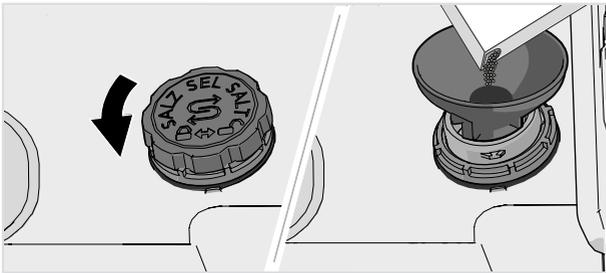
1. Remove the salt compartment lid by turning it anticlockwise.
