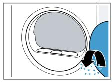
3. Remove the two-part fluff filter.
