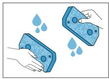
You can remove heavy soiling carefully using a vacuum cleaner. Do not clean the filter mat using cleaning products.
