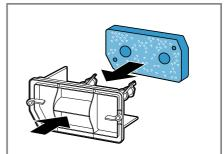
Ensure that the cleaned filter mat is not deformed, damaged or inverted when you push it onto the retainers.
