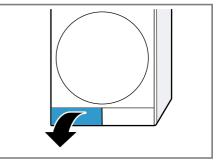
If you place a cloth beneath the maintenance flap, you can collect the remaining water from the base unit. 2. Open the lever for the heat exchanger cover.
