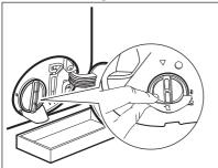
**4.** Turn the filter 180 degrees in anticlockwise direction to open it, without removing. Let the water flow out.
