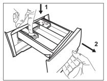
2. Remove the top part of the additive compartment to aid cleaning. Make sure that all detergent residue is removed from the upper and lower part of the recess. Use a small brush to clean the recess.
