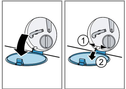
5. Slide a sufficiently large container under the opening.
