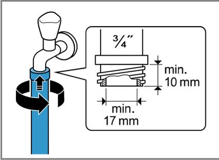
3. When connecting to a 21 mm = 1/2" tap, first fit the adapter with a sealing washer.
