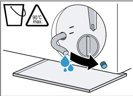
8. Firmly press on the sealing cap.
