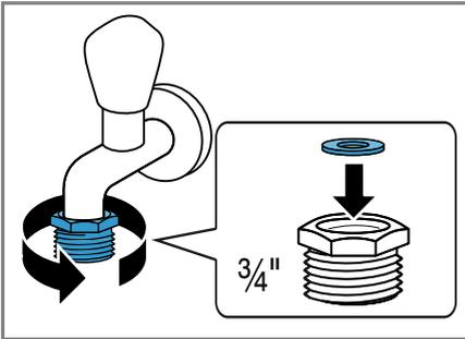
4. Open the water tap carefully and check that the connection points are tight.
