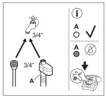
Connect the other end of the COLD water inlet hose to the cold water tap with 3/4" thread.
