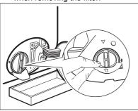
**4.** Turn the filter 180 degrees in anticlockwise direction to open it, without removing. Let the water flow out.
