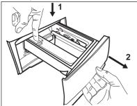
Remove the top part of the additive compartment to aid cleaning. Make sure that all detergent residue is removed from the upper and lower part of the recess. Use a small brush to clean the recess.
