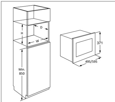
The microwave can be fitted in position A, B, C or D:
