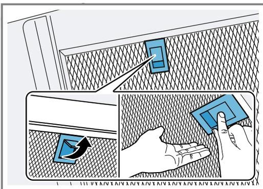
2. Remove the grease filters from the holders.
