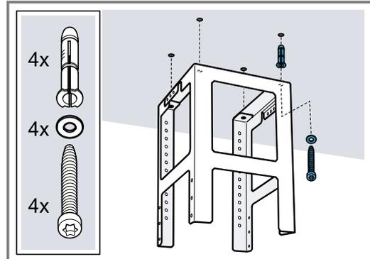
4. Drill four holes with a diameter of 8 mm to a depth of 80 mm for fastening the appliance and push in the wall plugs flush with the wall.
