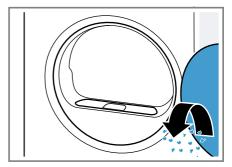
3. Remove the two-part fluff filter.
