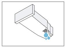
Check the condensation container filter regularly and clean the filter if it is dirty.  $\rightarrow$  *Page 35* Make sure that you insert the condensation container before operating the appliance.  $\rightarrow$  *Page 31*
