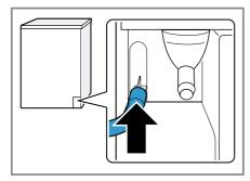
Push the water outlet hose as far as it will go into the connecting piece.
